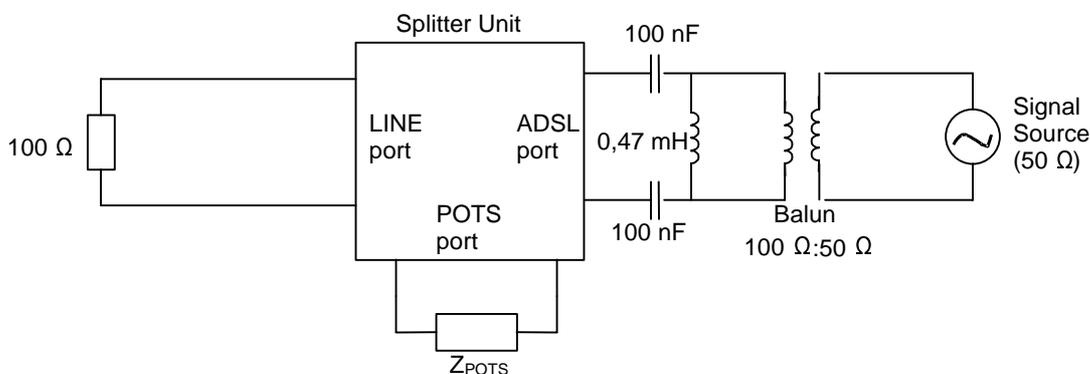
**Figure 7: Example ADSL to LINE insertion loss test setup**
