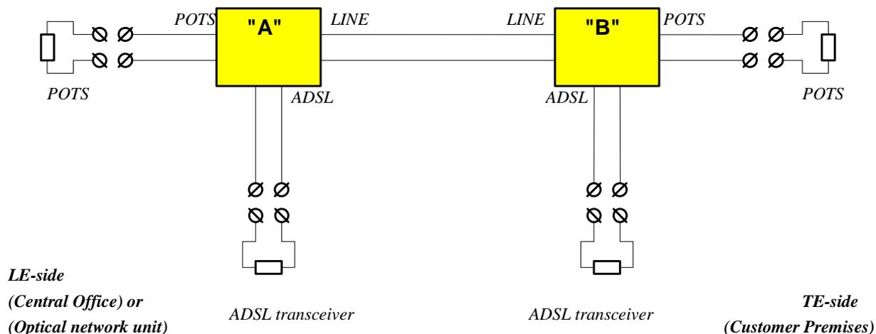
**Figure 1: Functional diagram of the DSL splitter configuration**
