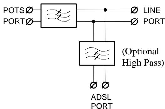
**Figure 2: Structure of the ADSL splitter filter**
