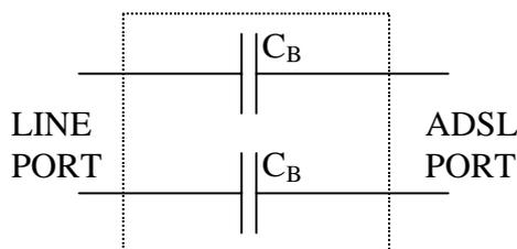
**Figure 3: Implementation of 1<sup>st</sup> order high pass filter**
