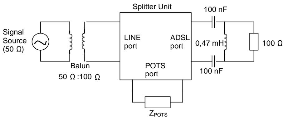
**Figure 8: Example LINE to ADSL insertion loss test setup**
