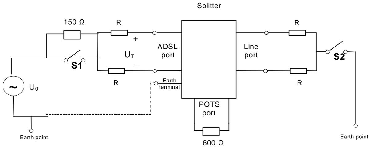
NOTE 1: The dotted circuit is only used if the splitter has an earth terminal.
