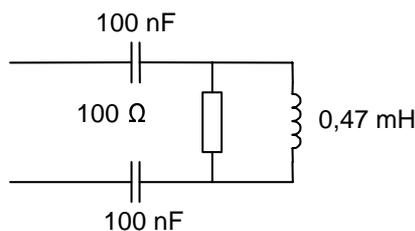
**Figure 5: Schematic diagram of the  $Z_{ADSL-M}$**
