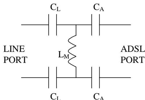
**Figure 4: Implementation of 3<sup>rd</sup> order high pass filter**
