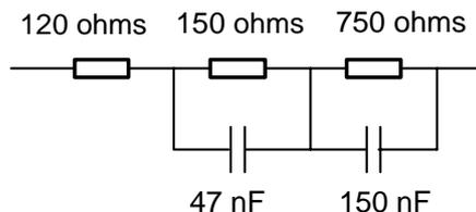
**Figure 6: Impedance  $Z_{\text{RHF}}$**
